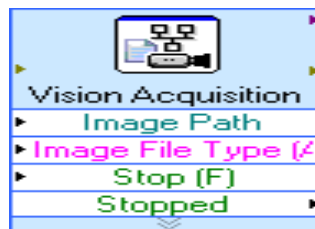
Figure 1: Vision acquisition function appearance in labVIEW VI
